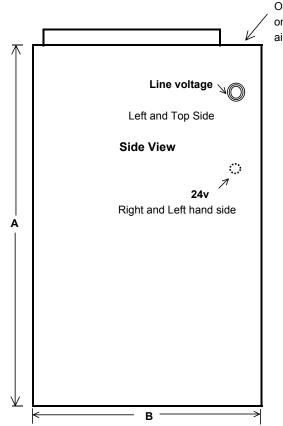
Optional line voltage on top or Left side of air handler.
